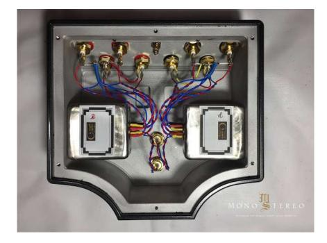
Only the secondary windings are made out of silver with one clear goal in mind. Better tone quality! Many listening tests were conducted to validate this particular decision. In the step-up transformer, up to 70-80% of the windings are "secondary windings" and in the Clinamen Silver Line, the bigger sections of primary windings are made out of copper wire.
