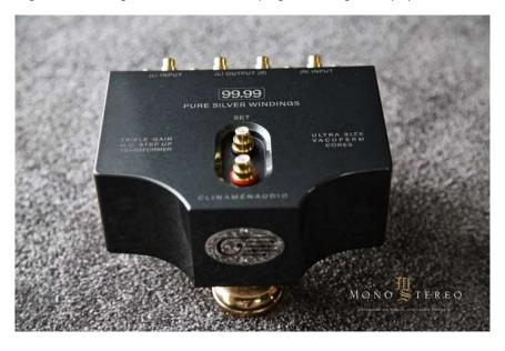
Stefano believes how any switch/selector that commutate primary will lower the sound quality and cause unwanted decay. This is why three different and independent primary windings are connected to the dedicated RCA connectors.
