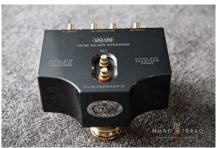
Another unique and shared feature of all Cliname Audio step-up transformer is the dedicated "harmonizing network" connector. This optimizes the electrical interfacing between the step up and the audio chain where it's inserted. (MC cartridge + step-up + pre-phono are the variables that occur to design the networks in question).
